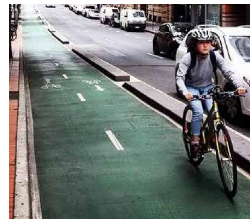
BI-DIRECTIONAL CYCLE LANE & SEGREGATED CARRIAGEWAY
