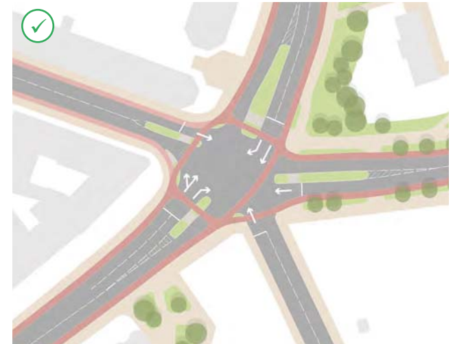
Vision of a protected intersection to improve the safety of pedestrians and cyclists. Note: the diagram is for illustrative purposes only.
