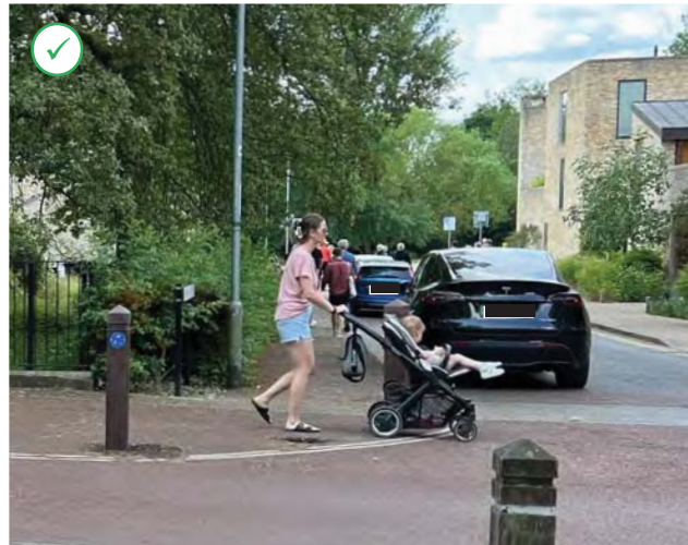
Example of raised table crossing from Accordia Cambridge
